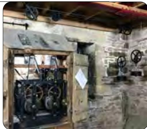
The clock will still require periodic attention to correct the time and adjust pendulum, the latter being made of wood and is affected by the ambient humidity.
